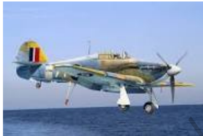
A HAWKER SEA HURRICANE WITH ARRESTER HOOK DEPLOYED, READY TO LAND. Photo : Wikipedia.
