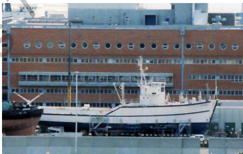
MV Madiba ex SAS Pretoria on a Synchrolift berth at Simon’s Town Dockyard.
